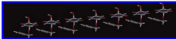
Figure 2. X-ray structure of monobenzyl-protected diketopiperazine made from serine. Cyclic amide-to-amide hydrogen-bonding is seen at the top of the array.
